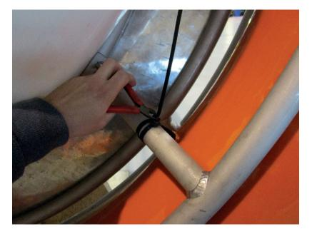
Cut the excess length of each cable tie- be aware of sharp ends.
