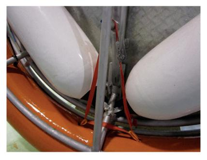
Fix the bottom lashing belt and tighten it to lift the two quarters in to place.
