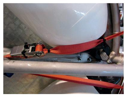
Secure the lashing locks with two 150mm cable ties.
