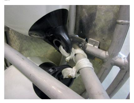
Mount 2 fenders with 6mm nylon rope as shown on picture, make sure the valves are pointing towards eachother. Then fix the other end of the fenders.
